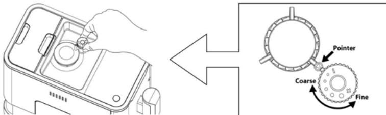
1. Only turn the knob for adjustment when grinder is in operation. Caution: Never adjust the grinding when the grinder is not operating. It can damage the grinder.
