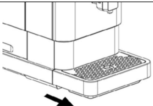
2. Drain the drip tray over sink and wash it with fresh water. Dry it afterwards.
