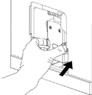
11.Place the coffee grounds container on the internal drip tray and insert into its original position.
